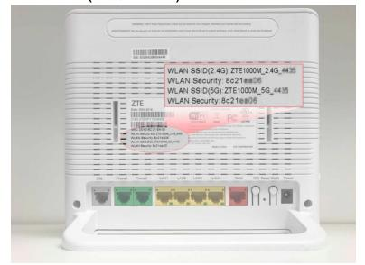
Wireless information (SSID/Password) located at the back of ZTE H268A Unit
